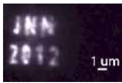
Fig. 1: “JNN 2012” pattern assembled during the JNN lab class by Single-Molecule Cut & Paste from approximately 700 DNA oligonucleotides labeled with Atto647N fluorophores.
