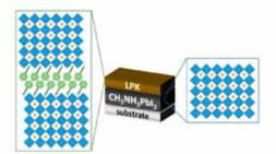
Schematic representation of a hybrid perovskite film composed of a MAPI/LPK bilayer.
