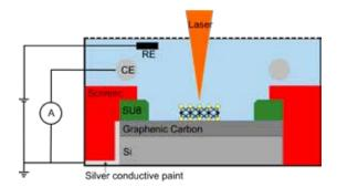
Electrochemical cell consisting of a graphenic carbon substrate covered with an electrically insulating photoresist (SU8). A 100  $\mu$ m diameter window enables the contact between electrode and electrolyte and the positioning of single MoS, flakes with known geometry.
