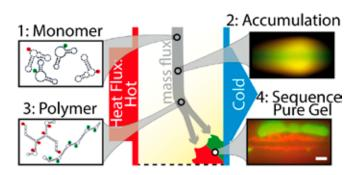
DNA strands that can fold into multiple hairpins are selected against their imperfect siblings with single base mutations by their gelation in a thermal trap. Slight sequence differences within the gel-forming strands lead to their separation into spatially distinct, sequence pure oligomer gels.
