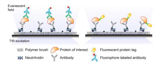
Figure 1: Schematic for single molecule immunoprecipitation.
