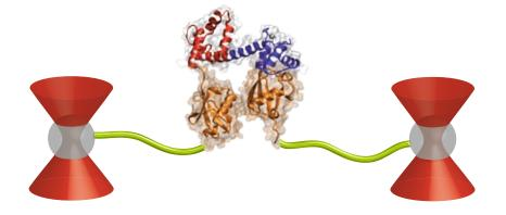
Figure 2: Zoom-in on the dumbbell configuration during the measurement. The protein is linked with ubiquitin-DNA hybrid handles (orange and green) to functionalized glass beads. Shown in red is the CaM N-domain, in blue the C-domain.
