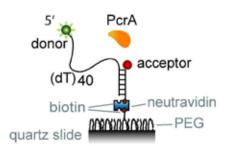
Figure 2: A partial duplex DNA is immobilized through biotin-avidin linkage on a PEG passivated surface to achieve specific binding. When PcrA protein is added with ATP on the immobilized substrate, single strand DNA was pulled through repeatedly resulting repeated sawtooth pattern in FRET signal. FRET is a molecular ruler that reports distance change between the two labeled positions.
