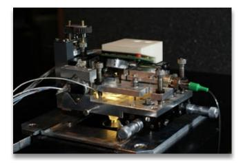
Figure 1: Experimental setup. The force-extension traces were recorded with a custom built AFM head specialized for long term SMFS data aquisition.
