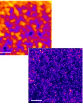
Fig. 2: Conventional confocal image of 20 nm fluorescent beads limited by the diffraction limit of light (upper left side) and corresponding super-resolved STED image of the same area (lower right side). Scale bars 1 µm.
