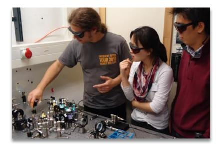
This module took the students through each step of aligning a self-built STED microscope. First it was shown how to select a certain wavelength range for the depletion beam using a prism-based monochromator and its importance for the success of the experiment was discussed. Furthermore the adjustment of the donut beam and its crucial contribution to the setup was explained and performed by using specialized components to analyze its circular polarization.
