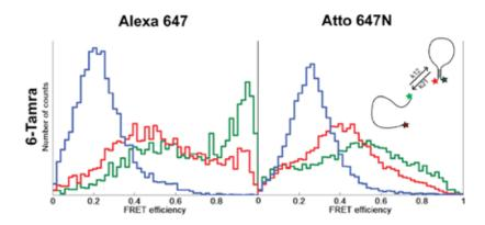
Figure 2: Exemplary comparison of DNA hairpin FRET efficiencies of selected dye combinations at NaCl concentrations of 10 mM (blue) 160 mM (red) and 320 mM (green).
