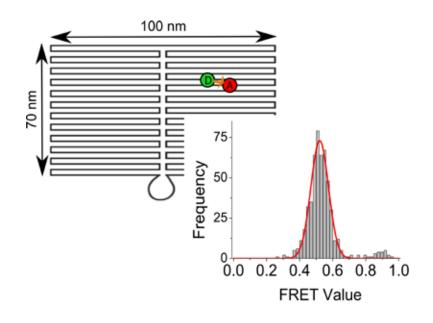
Figure 2: Scheme of a rectangular DNA origami with two incorporated fluorescent dyes.
