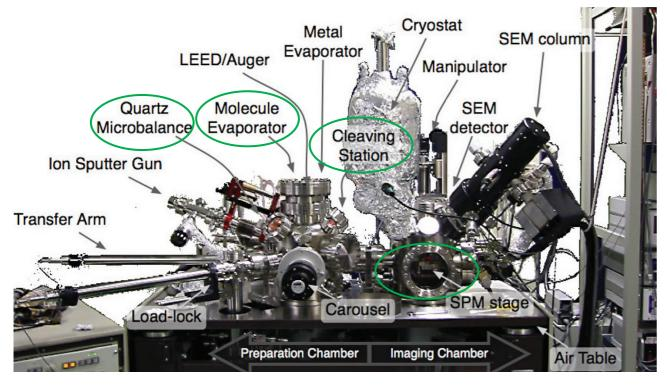
The JEOL JSPM 4500A Ultra-High Vacuum (UHV) Atomic Force Microscope (AFM) system.
