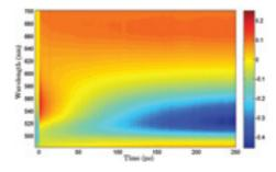
Figure 1: Absorption change in HPTS induced by a 400 nm pump pulse (colour bar represents the change in optical density).
