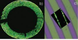
Fig. 1: Optical images of: a) Interdigitated bottom-contact device b) Green electroluminescence of PST-LET c) magnified contacts and localized light emission.
