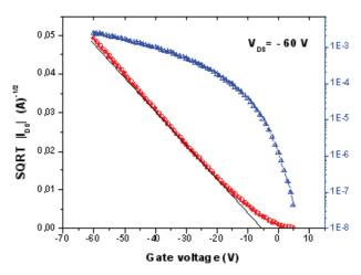
Fig. 4: Transfer characteristics of a PST-FET (deposition rate = 0.2 Å/s, nominal thickness = 18 nm,  $W/L=18800/40 \mu m/\mu m$ ).
