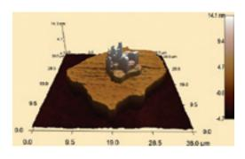
Figure 1: Height Image of a single multilayered domain.
