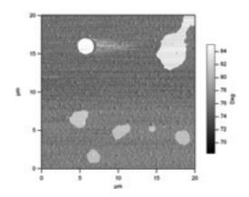
Figure 3: Phase Image of a growing sample, different contrasts expose different material stabilities.
