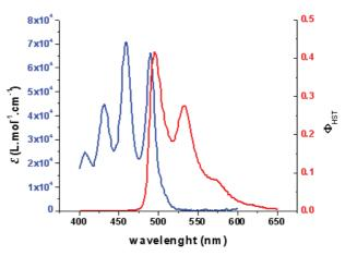
Fig. 3: The extinction coefficient and normalized fluorescence spectrum versus wavelength of PST molecule dissolved in 98% dichlorobenzene.
