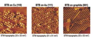
Fig. 3: The same molecule (1,3,5-benzenetribenzoic acid) was evaporated onto different substrates to study the influence of surface on the adsorption behavior. Apparently, the degree of ordering is heavily influenced. (a) copper, (b) gold, (c) graphite.
