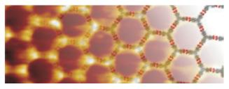
Fig. 1: Hexagonal pattern of a hydrogen-bonded self-assembled monolayer. Left side: STM image, right side: computer model. Cavities can be used to include guest molecules or metal clusters.
