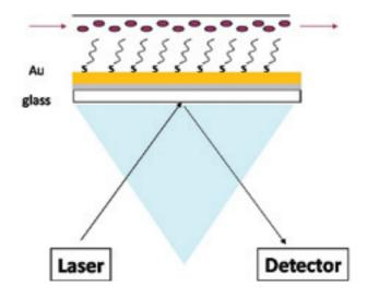
Schematics of an SPR measurement
