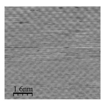
$10 \times 10$  nm atomic resolution image of the bare KBr substrate,  $\Delta f = -16$  Hz. New cantilever tips were prepared and baked overnight in preparation for the second stage of the experiment, and swapped and aligned the next day by students. 0.4 monolayers (ML) of PTCDI were deposited on the KBr using the molecular evaporator (Kentax). The sample was then imaged again by NC-AFM, and the island growth behavior of PTCDI on KBr was observed.
