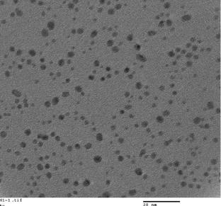
Figure 2: TEM of HS-(CH)15-CH3 capped gold nanoparticles synthesized at 80°C.
