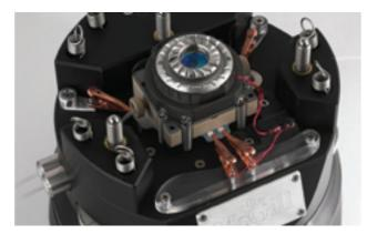
Figure 1: A zoom in of the electrochemical liquid cell
